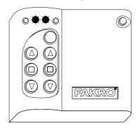
**5\***. Programming error – two middle LEDs flashing for app. 2-3 sec.
