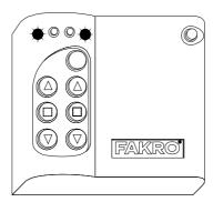
**5\***. Programming error – two external diodes flashing for app. 2-3 sec.
