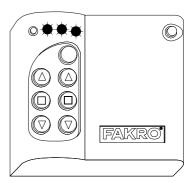
**6\***. Programming error – LEDs flashing for app. 2-3 sec.).
