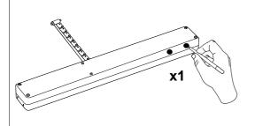
**4.** Press "P" button on the device and hold it for 0.5 sec. (see Device Programming Manual).
