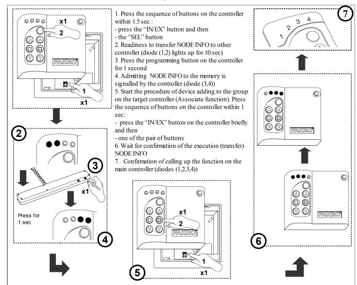
**Note!!!** In the new version of the controller, stopping of any procedure is possible by pressing of "IN/EX" buttons. In older version, it is necessary to wait 10 sec. until the moment of signalling the error by the controller or resetting it by removing the batteries.
