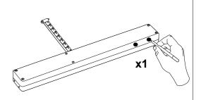
3. Press "P" button on the device and hold it for 0.5 sec. (see Device Programming Manual).
