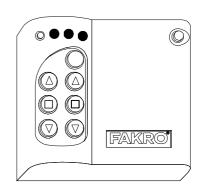
**3**. The controller is signalising readiness for device deleting (three LEDs on for 10 sec.).
