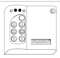
2. The controller is signalizing its readiness for excluding the device from the network (two middle LEDs on for 10 sec.).
