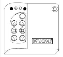
4. The controller is signalizing that the device has been excluded successfully (two external diodes on for app. 2-3 sec.).
