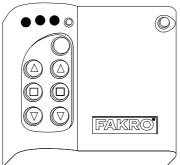
**5**. The controller is signalizing successful device deleting (three LEDs on for app. 2-3 sec.).
