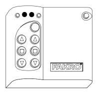
**4**. The controller is signalizing that the device has been successfully added to the network (middle LEDs on for app. 2-3sec.)
