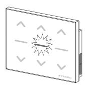
**5\***. Programming error – button flashing for 2-3 sec. as presented in the drawing.
